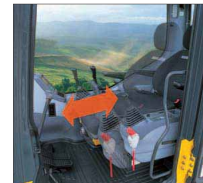
Seat Sliding Amount: 340 mm 13.4", increased 120 mm 4.7"
